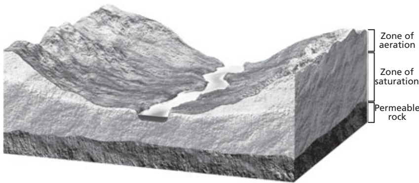
Groundwater soaks into the ground, passes through the zone of aeration, and collects in the zone of saturation.
